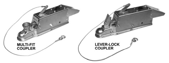
Surge braking is accomplished by replacing a trailer's standard tongue coupler with an actuator and adding hydraulic brake assemblies. The "surge" or "push" of the trailer toward the tow vehicle during deceleration automatically synchronizes these trailer brakes with the tow vehicle brakes. As the trailer pushes against the vehicle, the actuator telescopes together and applies force to its master cylinder, supplying hydraulic pressure to the trailer's brakes.
