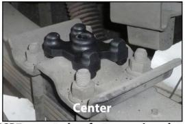
**PSP7** mounted on factory spring plate
