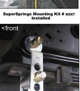
front ~ spring eye bolt threads out
