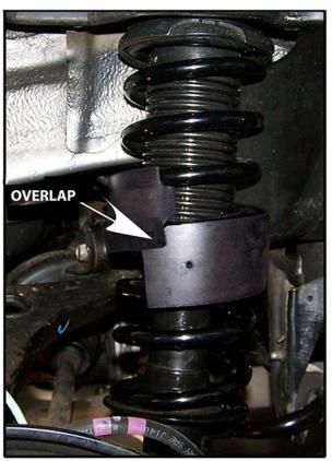
Installed on a 2011 Outback To complete installation install nylon wire ties
