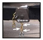
Note: The suggested starting point is to have three (3) full chain links showing under the latch. Do this on both sides of the trailer.
