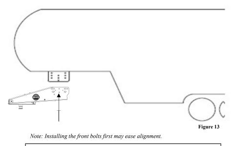
▲ <u>WARNING</u>: The 5<sup>th</sup> Airborne pin box is heavy, take care to maintain adequate support under the 5<sup>th</sup> Airborne arm until at least 2 bolts per side are installed. Failure to do so may result in death or serious injury.
