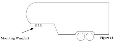
2. Remove the existing pin box, taking care to remove any necessary wiring and/or break away switch if attached to the pin box. (If removed, the break away switch must be reinstalled after installation is complete)
