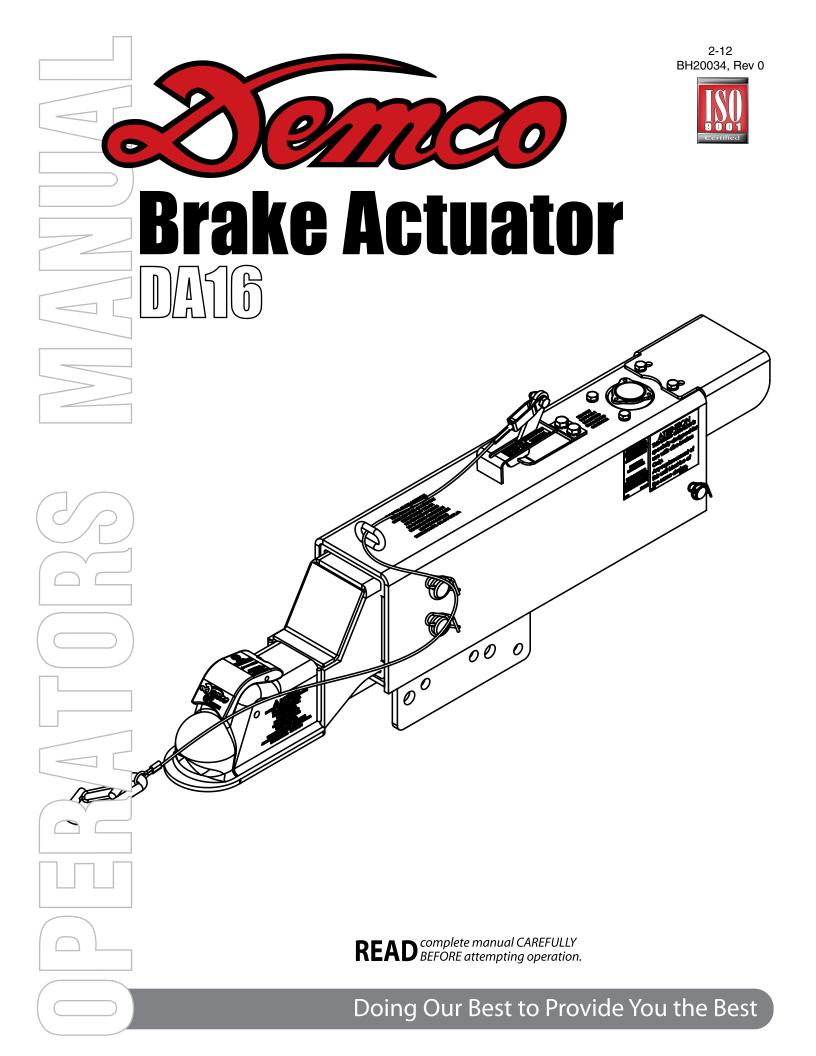
Model DA16 is a heavy duty surge brake actuator for trailers with two or four wheels. When brakes are applied on the towing vehicle, forward inertia of trailer toward towing vehicle applies brakes on trailer in direct relation to manner brakes are applied on towing vehicle. Brake towing vehicle hard and brakes on trailer are applied hard. Master cylinder push rod spring assembly protects system from hydraulic pressure overload.
