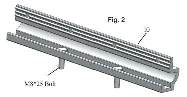
**3.** Place one Connecting Clamps (10) onto each end of the Side Rails (3). Install a third Connecting Clamp (10) in a position that will be suitable to connect Post A (1) and Post B (2) later. Secure them temporarily with Carriage Bolts and Lock Nuts from Bolt Set A. (Fig. 3)
